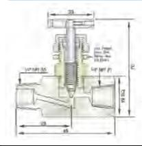
Sync-Lok Mini Needle Valves are also available in Female to Female, Male to Male & Male to Female end connections
