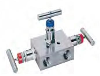
Sync-Lok 3 Valve Manifold Pipe to Pipe design for remote mounting, connecting system impulse lines and transmitters, This valve consist of 1/2" NPT Female connections on 2 1/8" (54mm) centers and one equalizer valve and two block valve.
