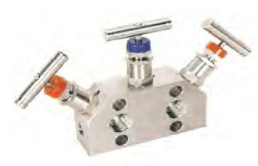
Sync-Lok 3 Valve Manifold Pipe to Flange, base mount connection design for connecting system impulse lines and transmitters, This valve consist of 1/2" NPT Female connections on 2 1/8" (54mm) centers and one equalizer valve and two block valves.
