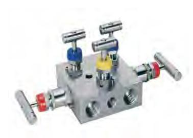
**Sync-Lok** 5 Valve Manifold Pipe to Pipe design for connecting system impulse lines and transmitters. This valve consists of 1/2" NPT Female connectors on 2 1/8" centers (54mm) to suit the inlet connection. This valve provides two instrument isolation valves, two equalizer valves and one bleed valve (for testing).
