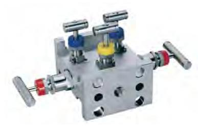
to Flange design for connecting system impulse lines and transmitters. This valve consists of two Flange connections with Teflon/Viton O-Ring packing on 2 1/8" centers (54mm) to suit the inlet connection. This valve provides two instrument isolation valves, two equalizer valves and one bleed valve (for testing).
